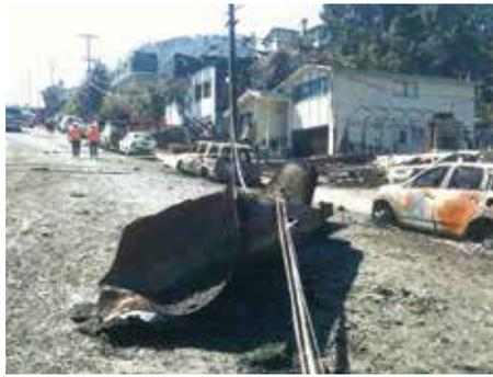
*The ruptured pipeline*
